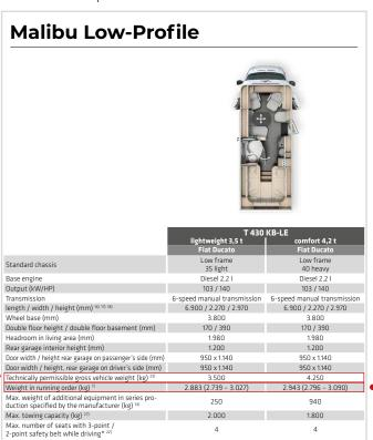
The technically permissible gross weight of the vehicle (e.g. 3.500 kg) must not be exceeded under any circumstances while driving. If the vehicle exceeds the technically permissible gross weight while driving, this constitutes a regulatory offence which may be punishable with a fine. We therefore urgently advise you to check this before each journey and ensure that you and your vehicle do not exceed the technically permissible gross weight (e.g. 3.500 kg).
